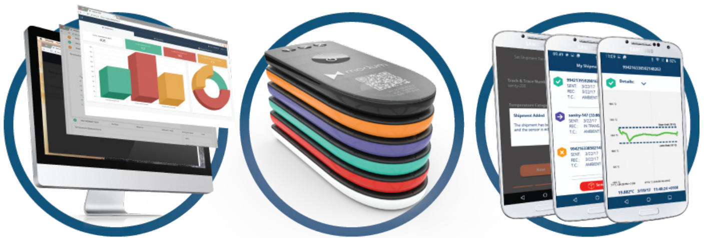
Figure 2: Components of the modum system: dashboard, temperature loggers, and mobile application
